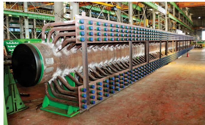
Primary Super Heater Outlet Header in fabrication
