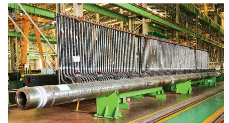
Economizer Inlet Header in fabrication
