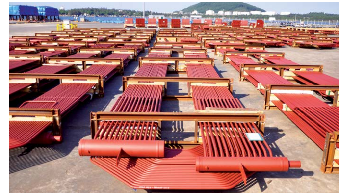
Coil Platen Super Heater ready for shipment
