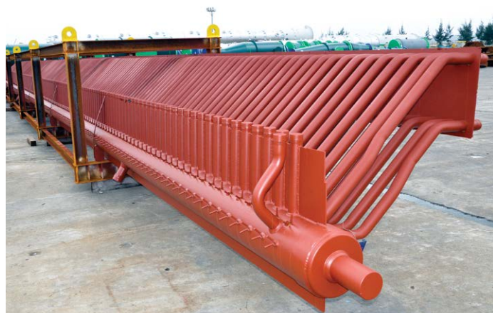
Packing Primary Super Heater Inlet Header
