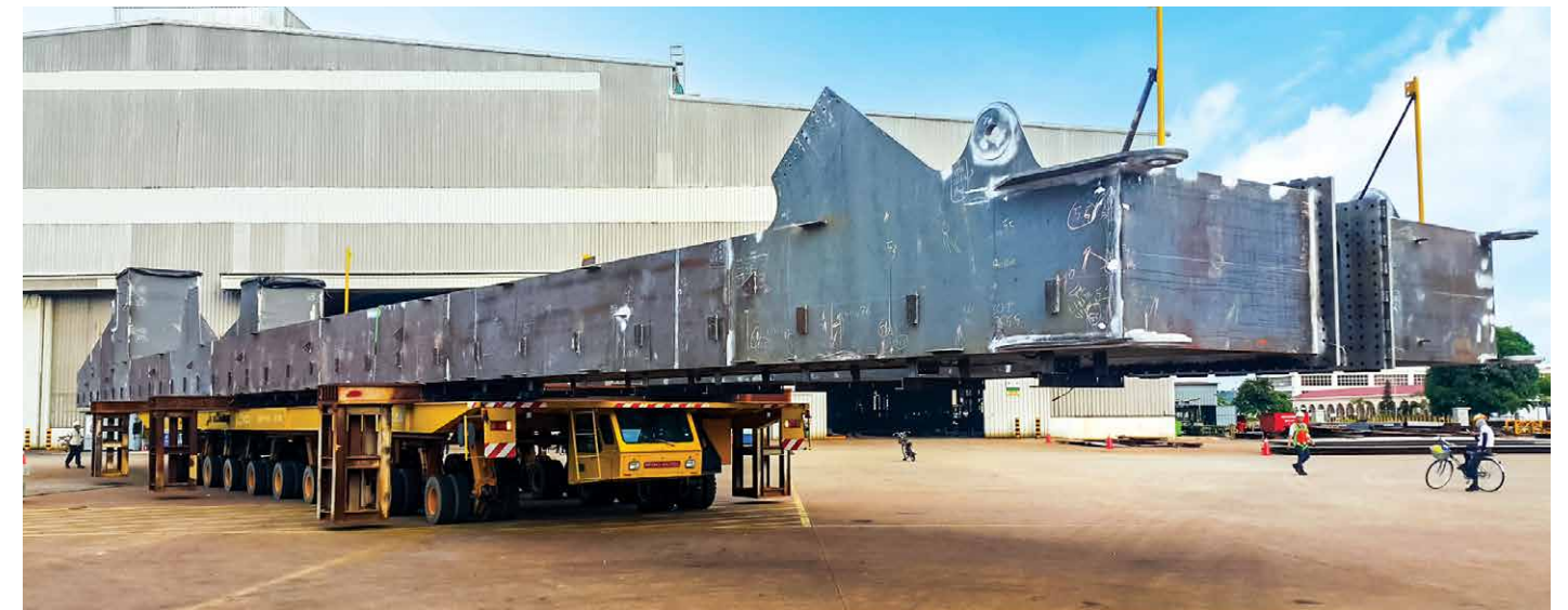
Parts of an RMQC being moved by an SPMT to Painting & Shot Blast
