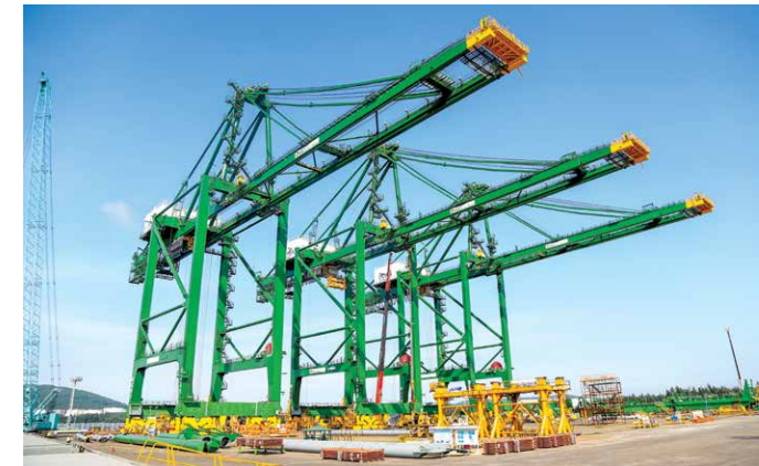
3 out of 12 Super Post Panamax Cranes for Bharat Mumbai Container Terminal (PSA), India
