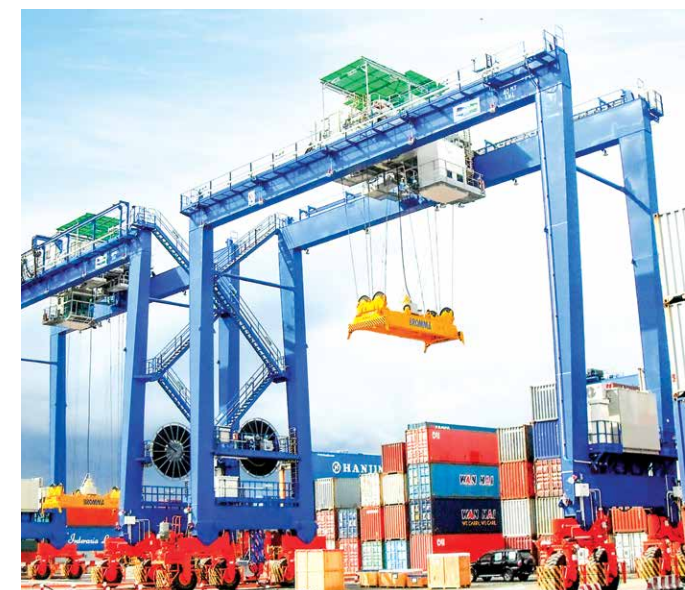
2 Rubber Tired Gantry Cranes (RTG) supplied to Sai Gon New Port, Vietnam
