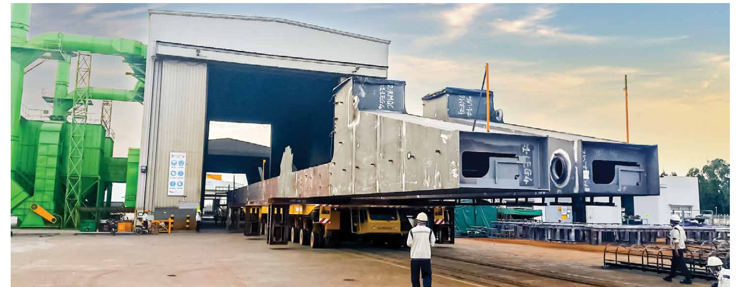
Parts of an RMQC entering the Shot Blast shop
