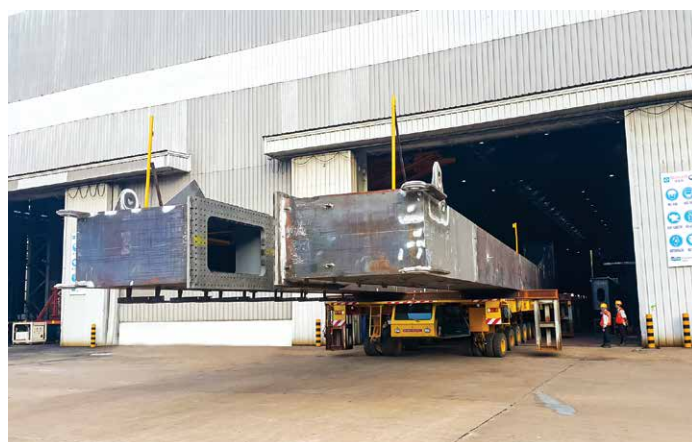
Parts of an RMQC are moved out of the indoor shop
