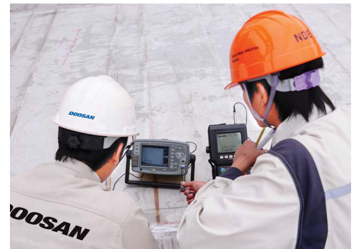
Steel is checked on arrival and during production
