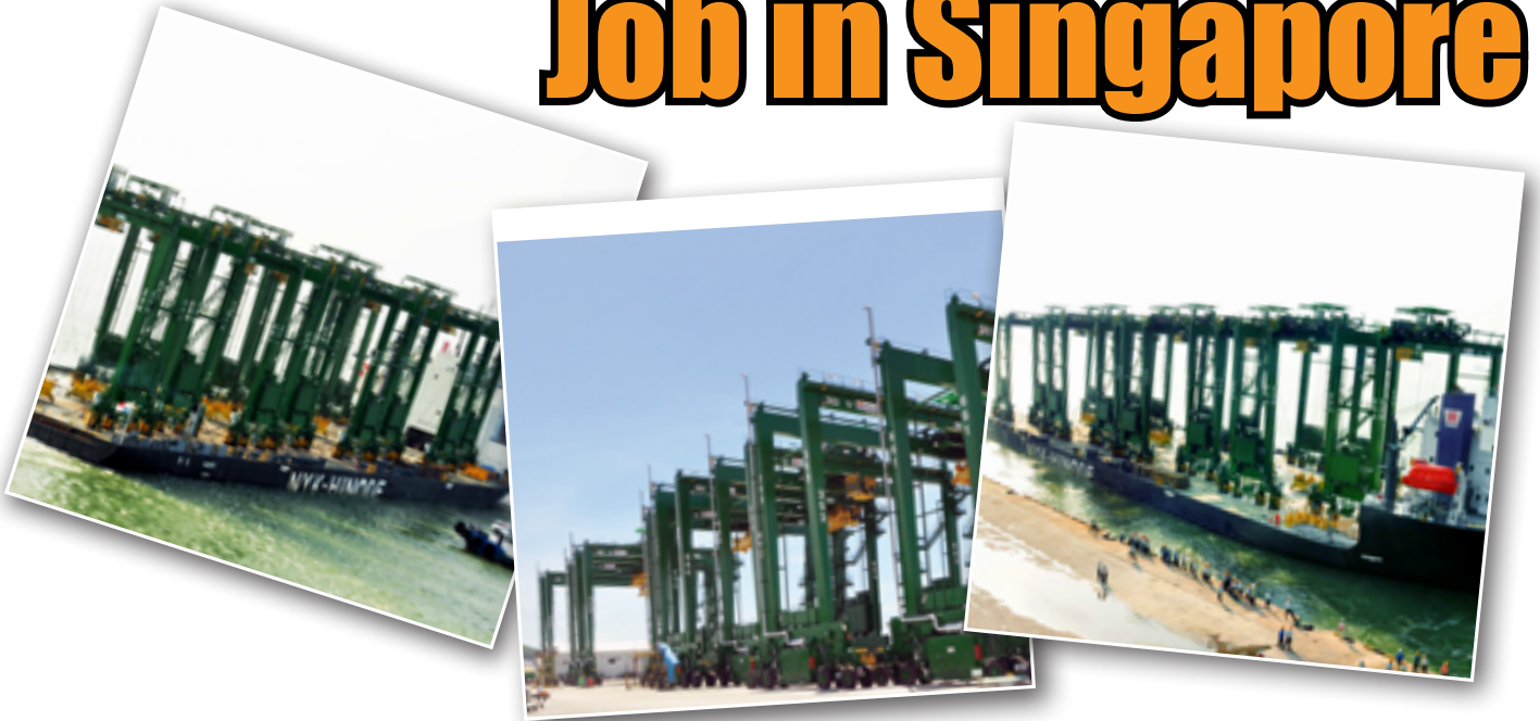
(The last group of eight Rubber Tired Gantry Cranes are loaded and depart for Singapore. These cranes have 16 wheels that can simultaneously rotate 360 degrees making them one of the most versatile cranes in logistics.)
