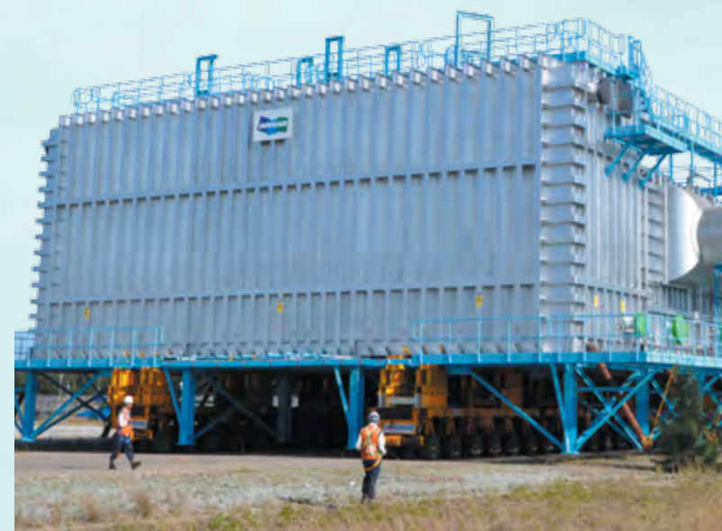
A 4,000 ton desalination evaporator moves to the port for shipment
