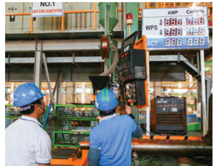
Visualization of a welders AMP's are displayed on an electronic board
