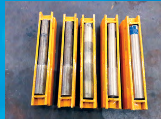
A Keson to prevent scratches during pipe turning
