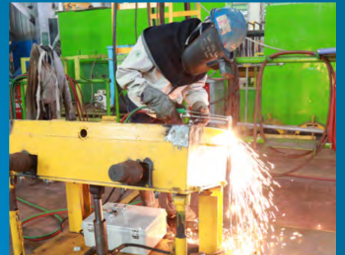
Vo Van Hung, Boiler Shop with automatic welding Keson which improved the UT test rate and increased production capacity
