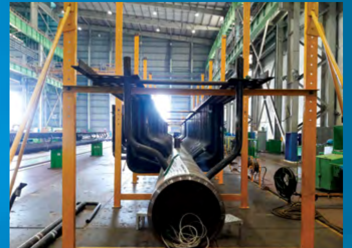
A multipurpose keson frame for fit up and welding
