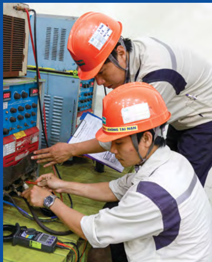
Checking the welding current to be sure it meets the requirements of WPS
