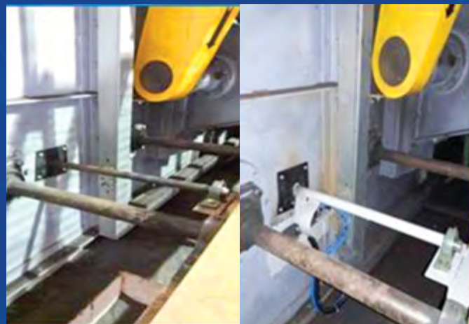
Pre-Keson Cleaning of products by sand and the after Keson Cleaning with the Blow Off system
