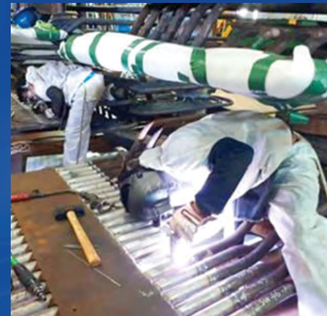
Welder's Keson chair supports the shoulder and reduces fatigue
