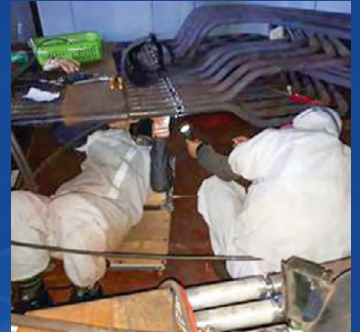
Welder's Keson chair supports the shoulder and reduces fatigue
